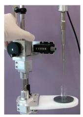
The crank is then turned to slowly raise the stand up the rod. When the probe begins to enter the Alignment Tool, you may need to adjust the position of the stand so that the probe is centered in the tool. Simply loosen the two thumb screws underneath the stand, use one hand to move the stand forward/backward and left/right until the probe is centered, then re-tighten the thumbscrews. You may need to refine the position again slightly when you test with a tube in the Tube Cooler (right).
